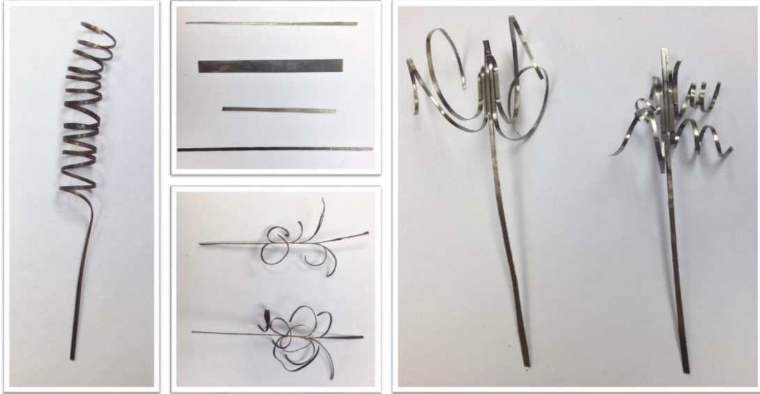
Figure 15. Unique whisker geometries used in an attempt to induce oscillations
