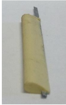
Figure 60. Galfenol Whisker with attached airfoil.
