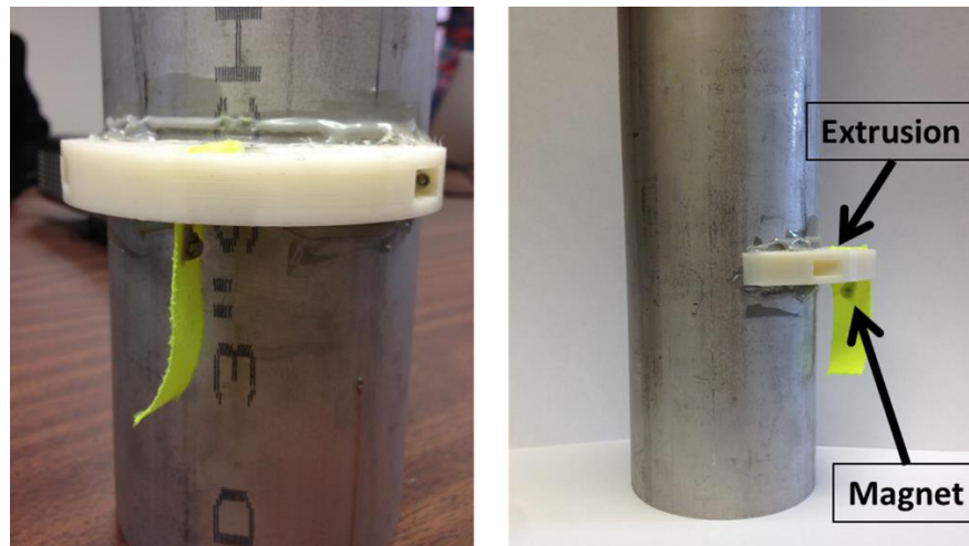
Figure 11. Photographs of a seaweed sensor with a holder for a vertical post
