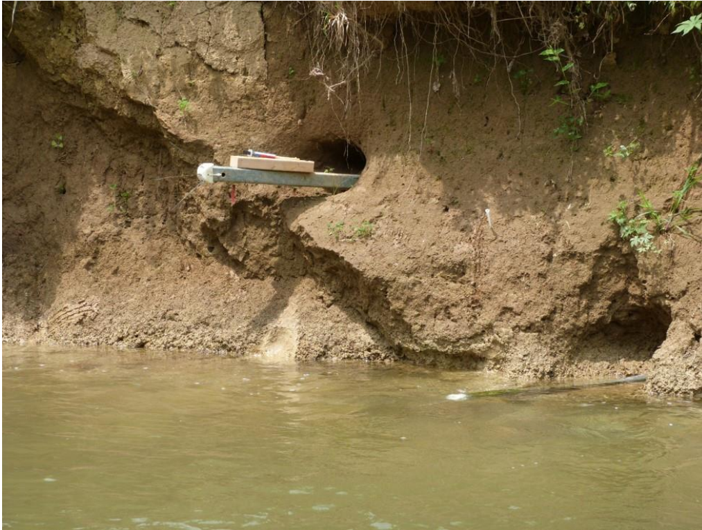
Figure 55. Whisker post caps attached to both the in-air and underwater posts via zip ties
